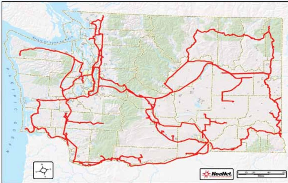
◀ The red lines across the State of Washington represent the NoaNet fiber optic backbone, largely available today (portions are to be built over the next two years), open to use by all. It is built as an advanced telecommunications infrastructure, capable of 10 gigabit Ethernet speeds. As such, the network is one of the fastest and most capable fiber optic networks available in the world today.
